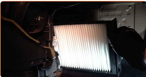
Utbyte: kupéfilter – RENAULT Megane II Hatchback (BM, CM). Tips:
