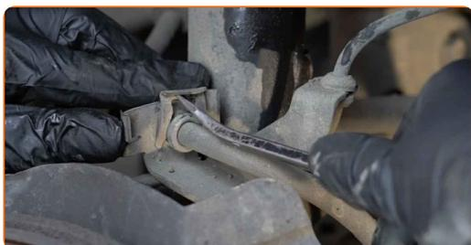
**18** Koppla loss ABS sensorns kablage.
